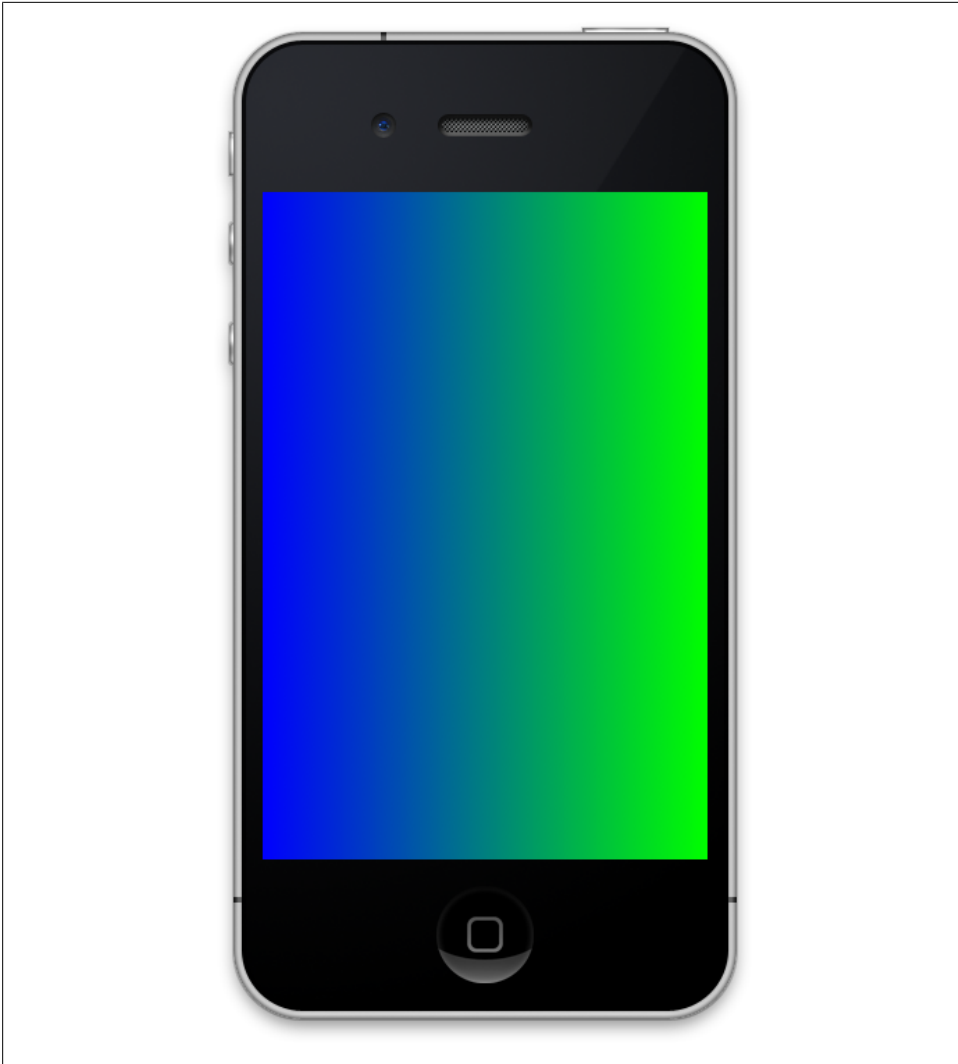
Figure 15-26. An axial gradient starting from the color blue and ending in the color green
